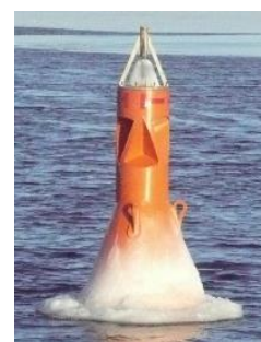
Figure 36 Radar reflector integrated into the buoy body
