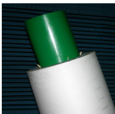
Figure 52 Radar reflector with plastic cover
