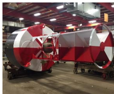
Figure 35 Radar reflector as part of the daymark
