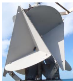
Figure 34 Radar reflector consisting of single corner reflectors mounted on a structure
