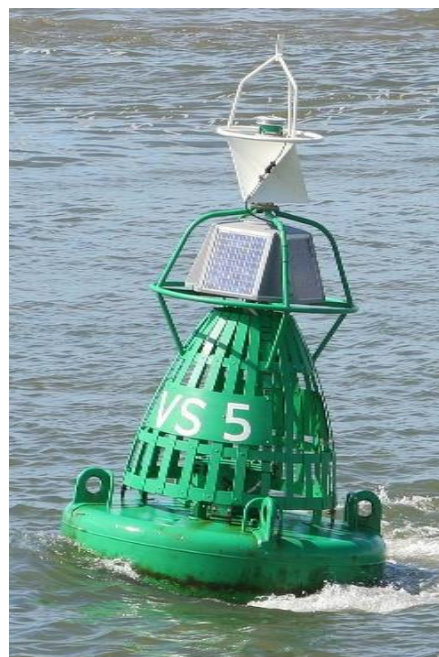
Figure 11 Steel buoy with radar reflector
