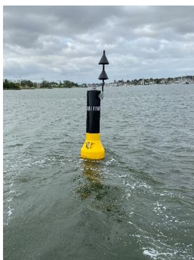
Figure 18 Plastic buoy with internal radar reflector
