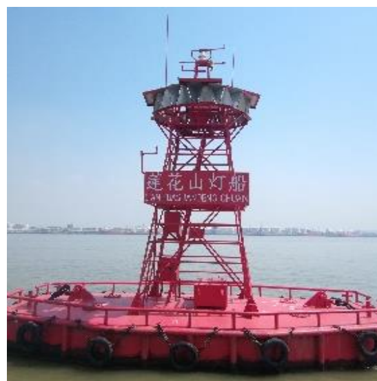
Figure 40 Corner reflectors on a LANBY
