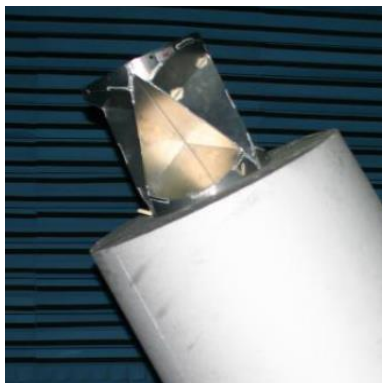
Figure 51 Radar reflector without cover
