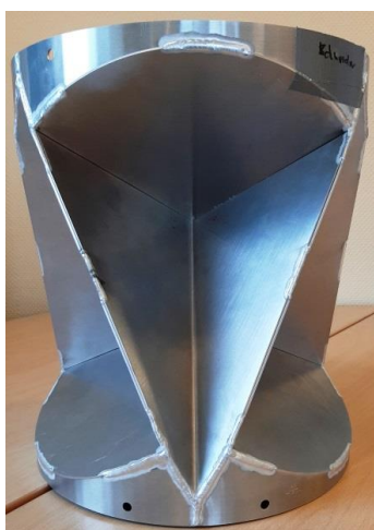
Figure 47 First sample of SR6-330 radar reflector
